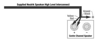
• If connecting a REL as a dedicated rear channel sub, connect the yellow wire to the left rear positive speaker terminal; connect the red wire to the right rear positive speaker terminal, connect the black wire to a ground lug or chassis screw. If the amplifier is of balanced differential design, please follow the instructions in the section above labeled Differential Connection.
